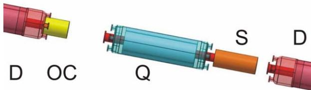
Fig. 5: Zoom of present HESR floor plan. D - dipole magnet, OC - orbit corrector, Q - quadrupole magnet, S - sextupole magnet. Not all He-covers and beam pipes shown. Further details will be added according to the progress of the project.
