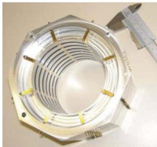
Fig. 3: Axial (top) and total (middle) view of the  $\lambda/4$  printed loop couplers. Bottom: Ring-slot coupler
