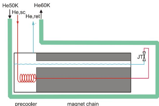
Fig. 6: Scheme of the cooling Helium flow through the cold mass
