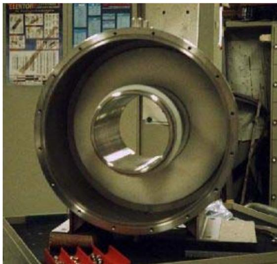
Fig. 2 Low-power barrier bucket cavity tank
