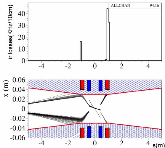
Fig. 5: Distribution (upper) and trajectories (lower) of particle losses at the IR with all machine collimators inserted. Rates are given for a 13mA bunch. The IP is at  $s=0$ .
