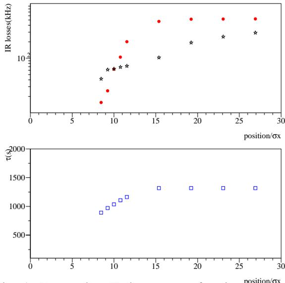
Fig. 4: Upper plot: IR losses as a function of the IR collimators openings measured in number of  $\sigma_x$  from the center of the beam axis. Black dots are losses downstream the IP, red dots are the upstream ones. Lower plot: corresponding Touschek lifetime.
