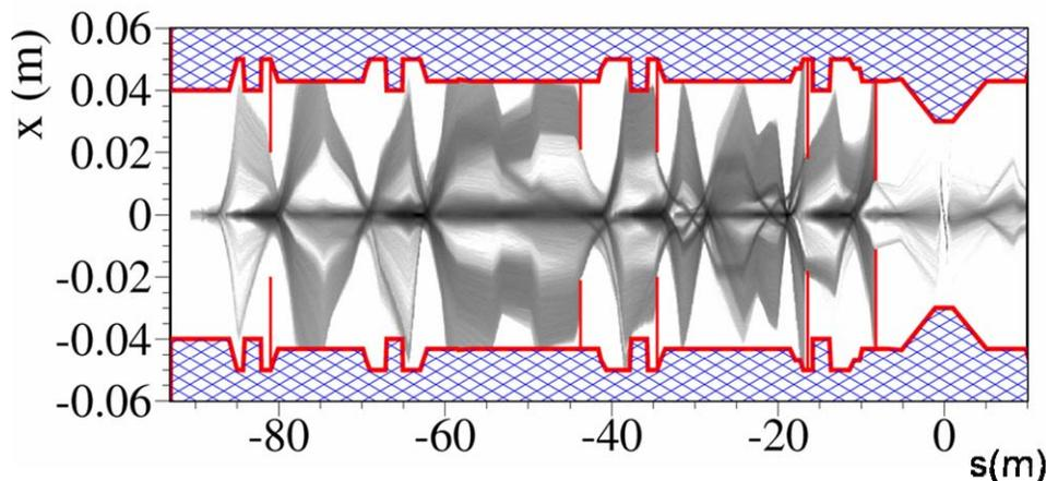
Fig. 2: Touschek particles trajectories plotted with all machine collimators inserted. The IP is at  $s=0$ .
