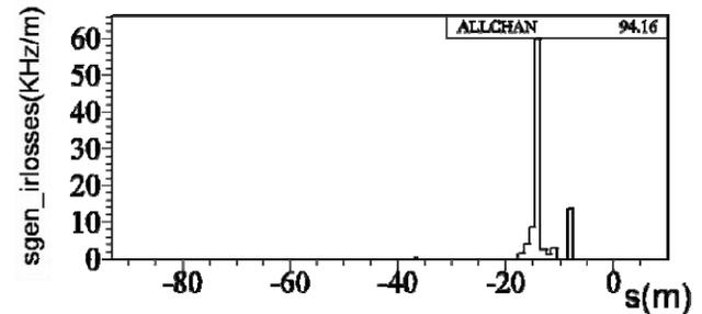
Fig. 6: Location source of Touschek particles getting lost at the IR, with insertion of collimators. Only particles generated in the last arc before the IR are still dangerous for the detector.
