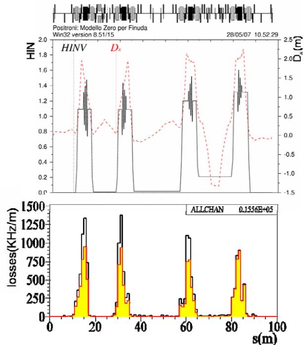
Fig. 1: Upper plot:  $H$  and dispersion functions for the DAΦNE upgrade optics. Lower plot: Distribution of Touschek scattering position for losses all over the ring or only at the IR, white and yellow histogram, respectively. The IP is at  $s=0$ .
