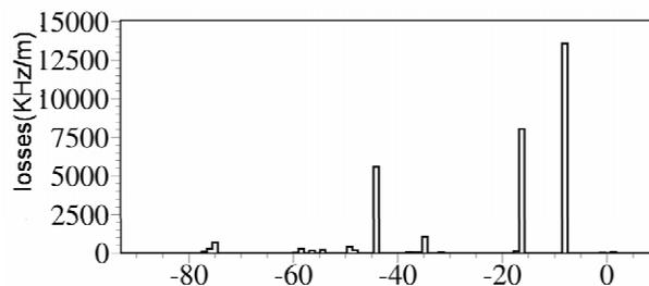
Fig. 3: Distribution of total losses plotted with all machine collimators inserted. The IP is at  $s=0$ .
