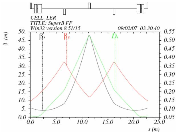
Figure 4: LER arc lattice cell.
