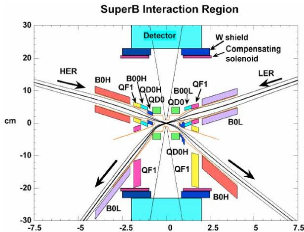
Figure 3: Interaction region for two asymmetric beams.
