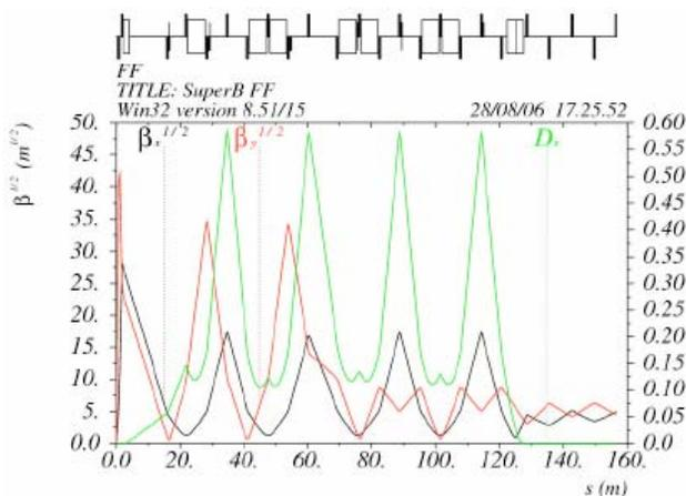
Figure 5: IR optical parameters for a Super-B-Factory.
