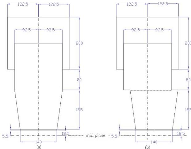
Figure 1: Drawing of a pole in the  $x$ - $y$  plane (a) before and (b) after the modification. The case refers to a pole where the particle is on the right of the vertical symmetry axis (geometric axis). Dimensions are in mm.
