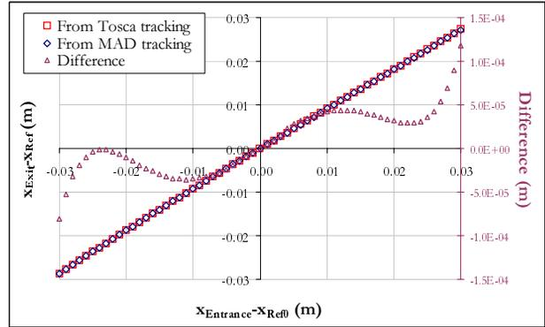
Figure 7:  $x$  exit as a function of the  $x$  entrance with respect to the reference trajectory. The difference is also shown.
