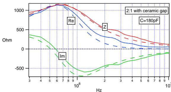
Figure 5: Impedance measurements and theoretical prediction assuming  $L(\omega)=[\mu'+(\mu'')^2/\mu']L_0$  and  $R(\omega)=\omega[\mu''+(\mu')^2/\mu'']L_0$ , where the complex permeability,  $\mu=\mu'-j\mu''$ , of Finemet® is known as a function of  $\omega$  and  $L_0$  is the core inductance in air, with packing factor and constant  $C$  of 180 pF.
