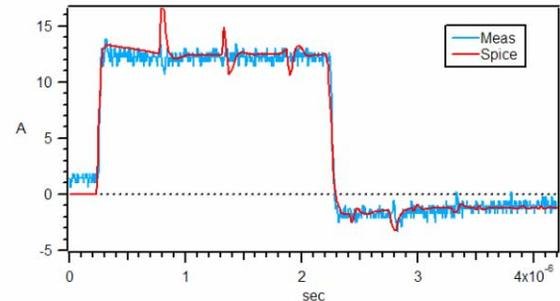
Figure 6: Matching resistance current ( $I$  in ampere) profile. Induced voltage  $V_{ind}$  is written by  $Z_M I/2$ , where  $Z_M$  (134 $\Omega$ ) is the matching resistance.
