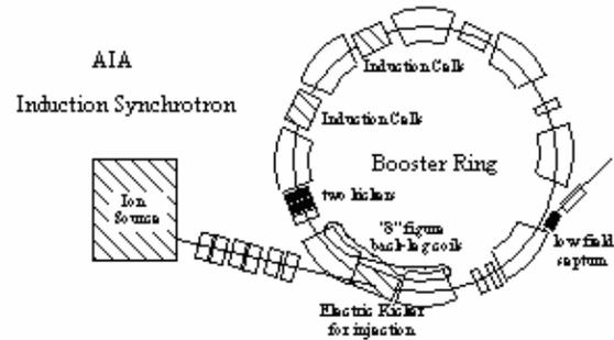
Figure 1: Schematic view of the KEK-AIA with the ion source and induction acceleration cells.
