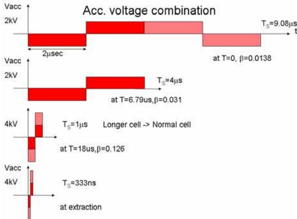
Figure 2: Acceleration scheme of the KEK-AIA from the injection to the extraction. A set of positive and negative pulse voltage is required for the magnetic core not to saturate. The pulse width must be changed during acceleration because the revolution frequency increases.
