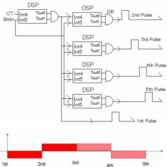
Figure 4: Trigger system of the KEK-AIA just right after the injection. Serial DSP array generates the timing signals to trigger the pulse voltages. The 1<sup>st</sup>~5<sup>th</sup> signals maneuver start/stop of positive/negative pulse.
