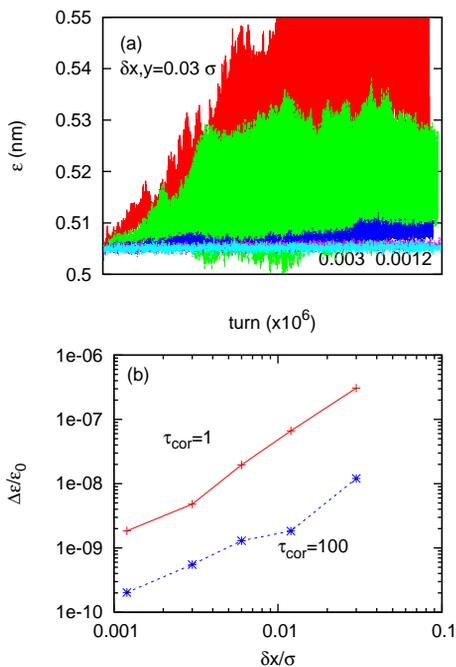
Figure 2: Emittance growth due to the fluctuation given by the strong-strong simulation.  $t_{cor}$  is the correlation time (turn) of the fluctuation.
