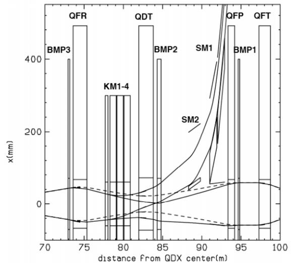
Figure 2: Injection beam orbit. Upper is from ref. [3]. Lower shows new version designed for low field of the SM2.
