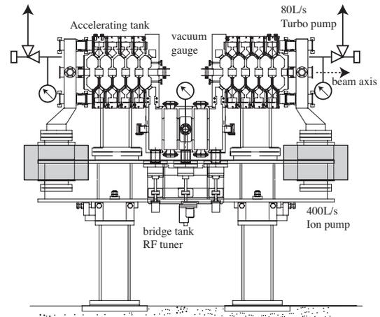
Figure 1: Schematic drawings of ACS buncher module.
