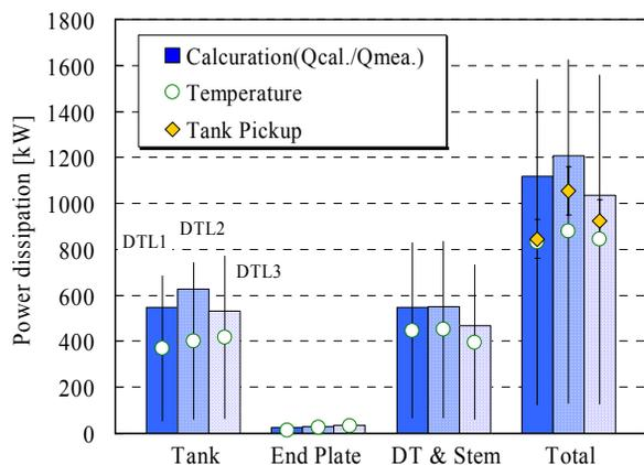
Figure 4: Power dissipation of the DTL
