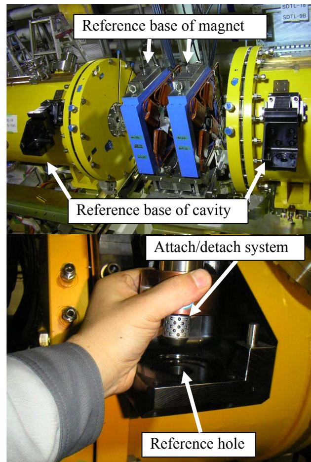
Figure 1: Reference bases of cavities and magnets, and attach / detach system for CCR holder.
