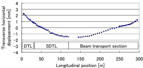
Figure 3: Horizontal position of the cavities and magnets in the straight section of the J-PARC linac.
