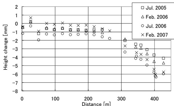
Figure 6: Height change of the accelerator tunnel since Feb. 2005
