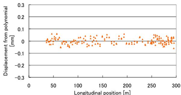
Figure 5: Transverse and horizontal displacement from the polynomial after the re-alignment.
