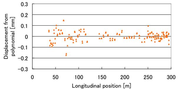
Figure 4: Transverse and horizontal displacement from the polynomial after the installation.
