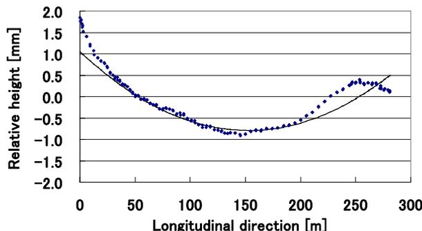
Figure 7: Relative heights of the DTL cavities and the quadrupole magnets in the linac straight section.
