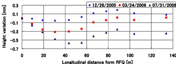
Figure 6: Height elevation of the vertical marker. Horizontal axis is the longitudinal position of the marker.
