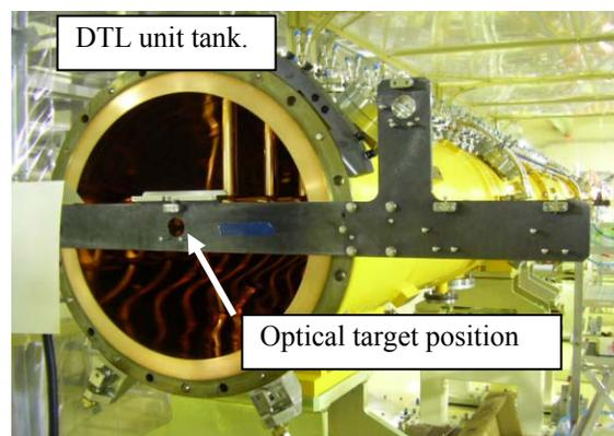
Figure 1: DTL unit tank and template for the alignment target holder.
