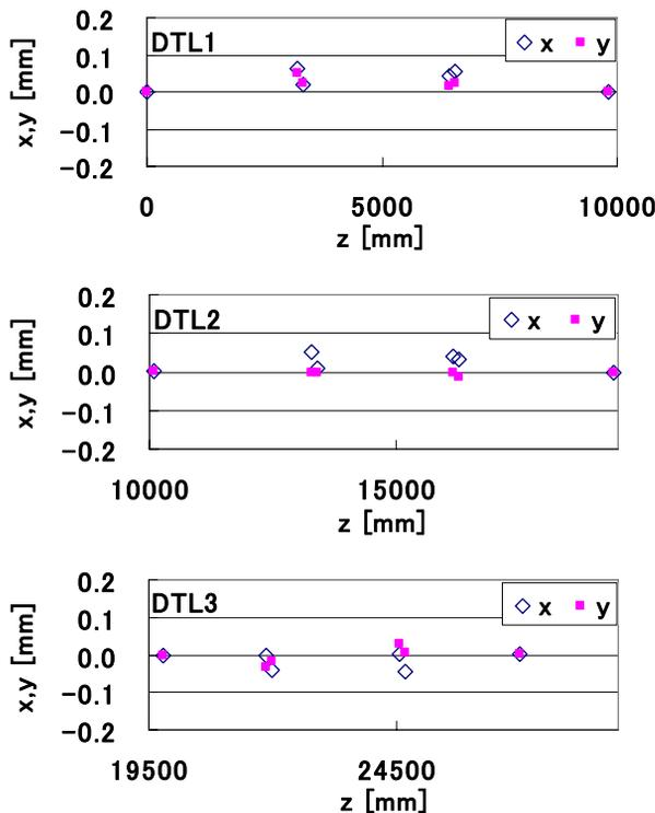
Figure 3: Displacement of unit tanks by docking for DTL 1, 2, and 3.
