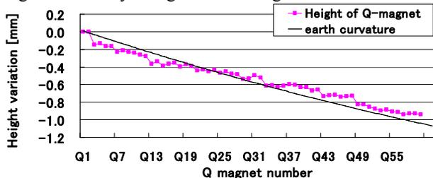
Figure 5: Relative heights of all magnets in the SDTL section. Dots are measured height and solid curve is the earth curvature.
