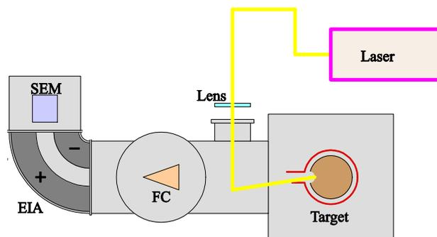
Figure 2: Overall view of the experimental setup.
