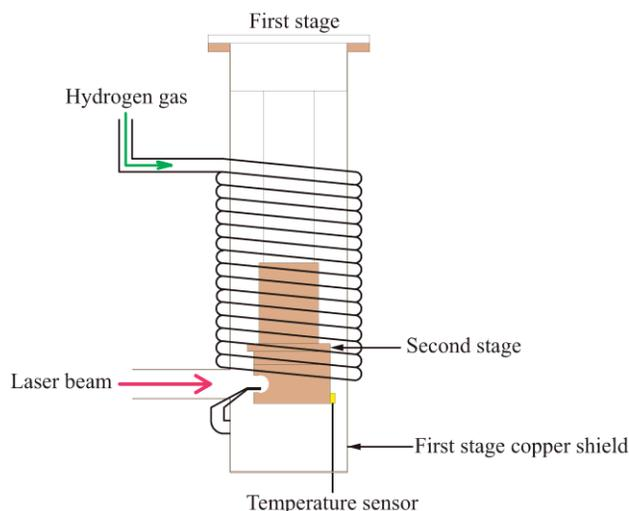
Figure 1: Solid hydrogen production equipment.
