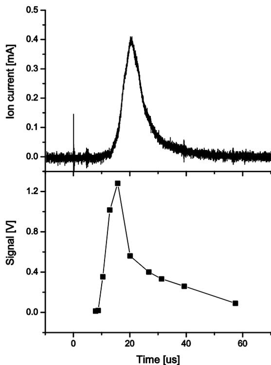
Figure 5: (Upper) Total ion current measured by the FC. (Lower)  $H^+$  ions measured by the SEM.
