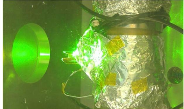
Figure 3: Half-wavelength Nd:YAG laser focused the solidified hydrogen target.
