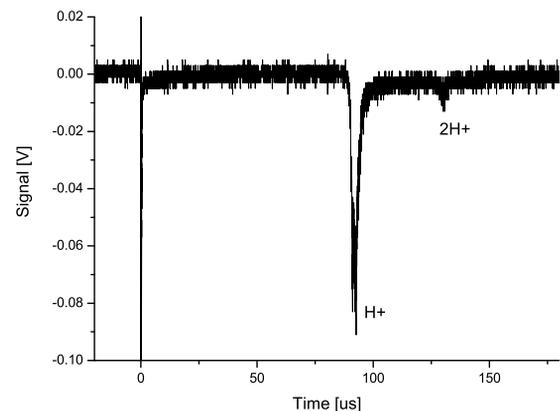
Figure 4: Peaks of  $H^+$  ions and  $H_2^+$  ions with the EIA voltage of 5 V.
