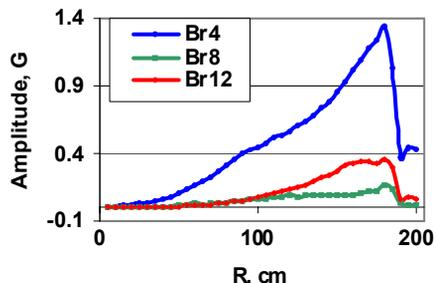
Figure 8: Dependence of amplitudes of harmonics of radial component on radii.
