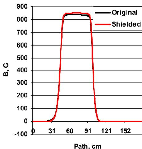
Figure 4: Magnetic field distribution along reference trajectory of beam motion.
