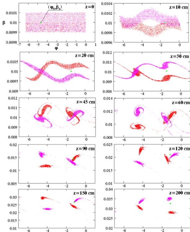
Figure 4: The bunching of the neutral dual beams.
