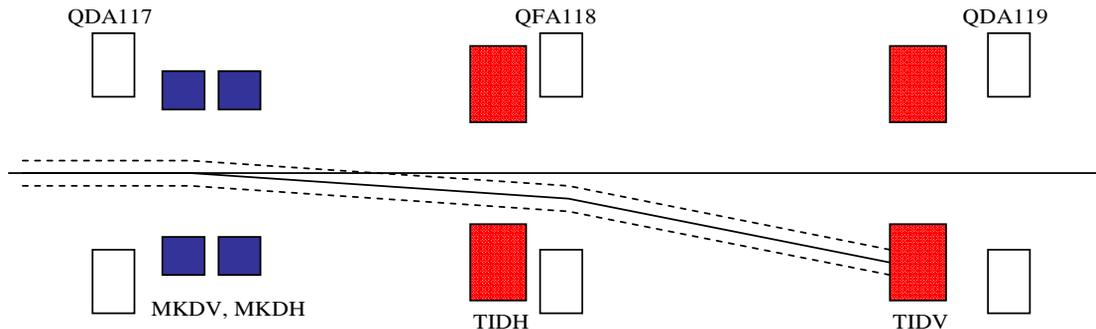
Figure 1: Schematic layout (side view) of the SPS beam dump system, showing the vertical and horizontal kicker systems (MKDV, MKDH) and the two beam dump blocks TIDH and TIDV.
