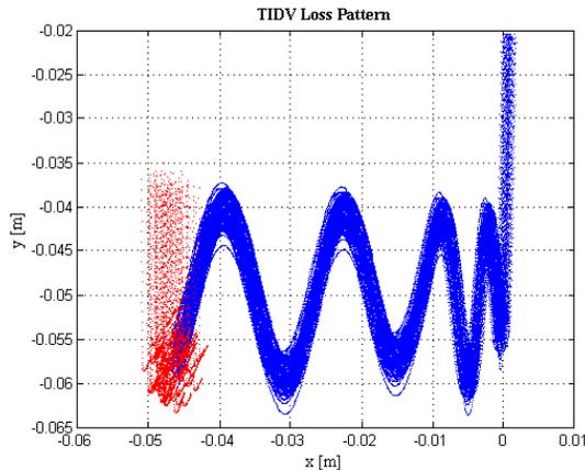
Figure 4: TIDV loss pattern, asynchronous beam dump (400 GeV, nominal pulse), blue: 1<sup>st</sup> turn, red: 2<sup>nd</sup> turn.
