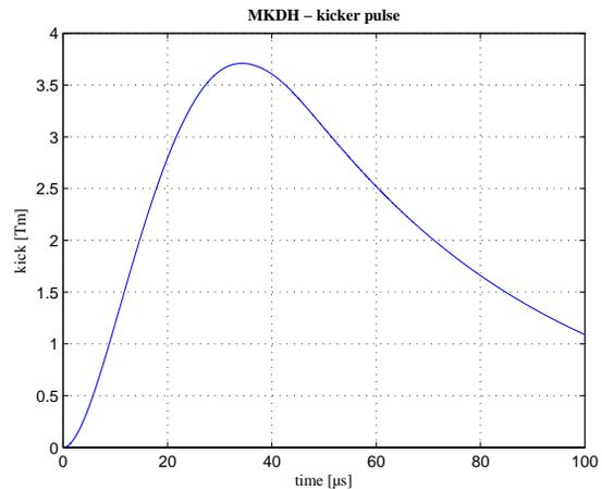
Figure 3: Simulated MKDH kicker pulse, 9 kV.
