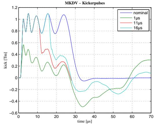
Figure 2: Simulated MKDV kicker pulses, 47 kV, nominal case (blue) and with sparks after 1, 11 and 16  $\mu$ s.
