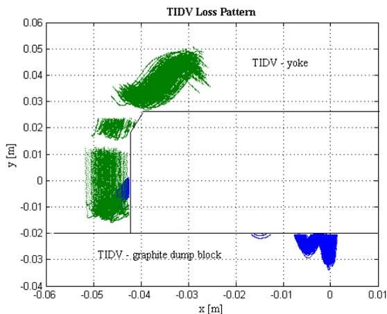
Figure 7: TIDV loss pattern, 400 GeV, short-circuit after 1 μs, blue: losses 1st turn, green: losses 2nd turn.
