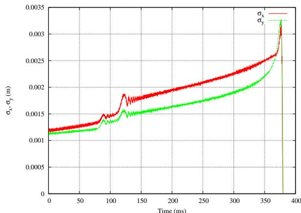
Figure 3: Evolution of the beam size at TCSG.A5L7.B1 after a powering failure setting the voltage to  $2V_n$  in RQ5.LR7.
