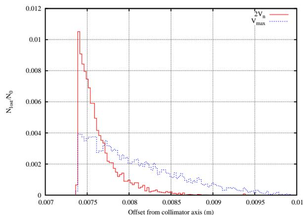
Figure 4: Distribution of the losses at TCSG.A5L7.B1 (right jaw) after powering failures setting the voltages to  $2V_n$  and  $V_{max}$  in RQ5.LR7. The half-gap of this collimator is 7.37 mm
