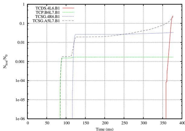
Figure 2: Distribution of the beam losses in different collimators after a powering failure setting the voltage to  $2V_n$  in RQ5.LR7.
