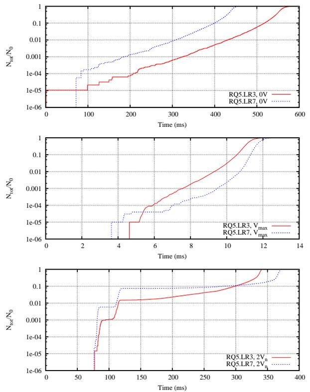
Figure 1: Beam losses as a function of time for the three cases of study: failure voltage set to 0V (top),  $V_{max}$  (middle) and  $2V_n$  (bottom).
