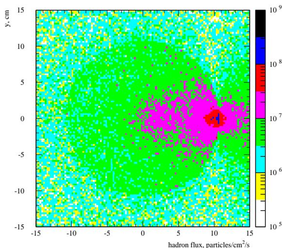
Figure 4: Hadron flux density, [particles/cm<sup>2</sup>/s] at the front surface of the TAN absorber in IR5, given for the rate of  $8 \times 10^8$  p-p inelastic interactions/s in the IP.
