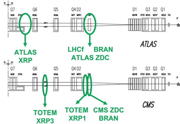
Figure 1: Very forward detectors in the LHC insertions IR1 and IR5 of the ATLAS and CMS experiments.
