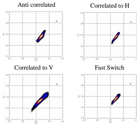
Figure 7: Single Particle Tune Diagrams at  $2.8 \times 10^{13}$  ppp.
