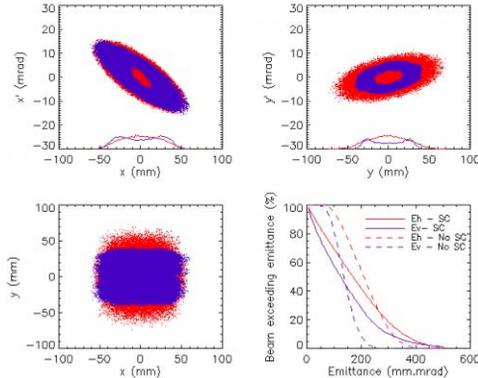
Figure 4: Phase space, Real space and Emittance occupancy of ISIS simulation at 0 ms with and without space charge.
