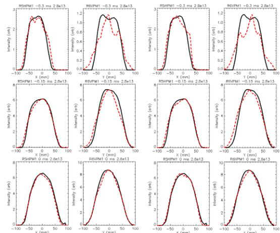
Figure 3: Measured (black) and Simulated (red) profiles at 3 machine time points. Left two columns, normal ISIS lattice. Right two columns, ISIS lattice with half integer driving terms.
