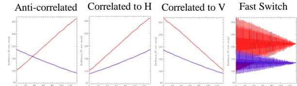
Figure 5. Centroid painting amplitudes over injection
