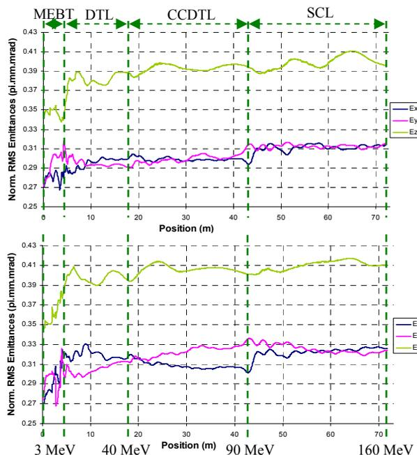
Figure 3: Longitudinal and Transverse Emittances evolution (Normalized RMS) in LINAC4 using RAL (top) and CERN (bottom) MEBT.
