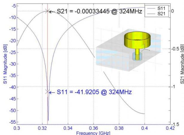
Figure 9: Doorknob transition structure simulation result.
