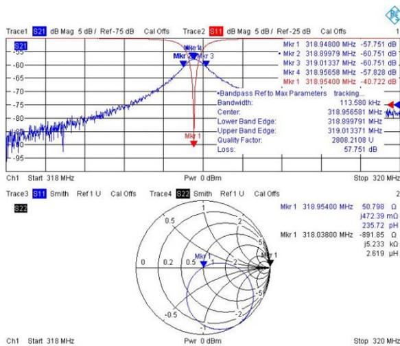
Figure 4: Braze RFQ critical coupling at about 319MHz.
