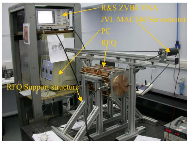
Figure 3: Braze RFQ cold model with end-plates on bead-pull experiment setup in Imperial College London.
