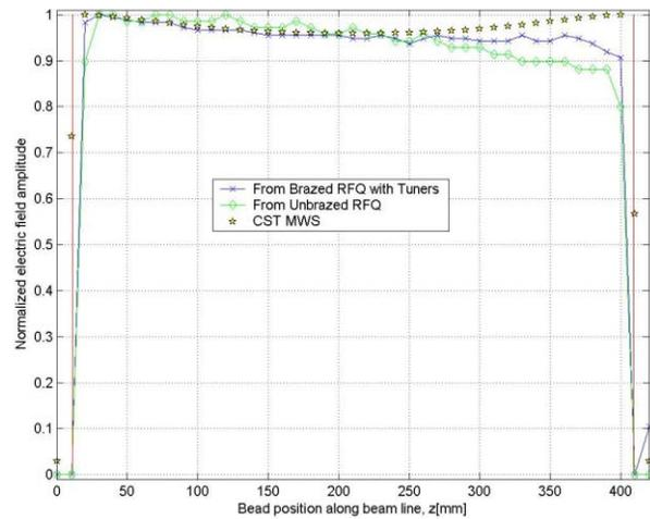
Figure 5: Electric-field distribution comparing between braze and unbrazed RFQ cold model with simulations.
