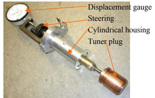
Figure 6: The mechanical tuner.
