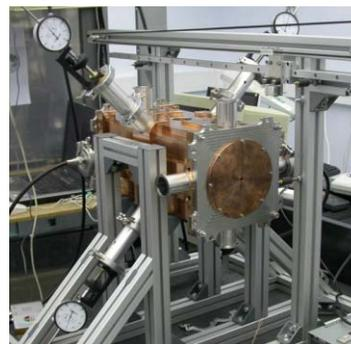
Figure 7: Mechanical tuners on braze RFQ.
