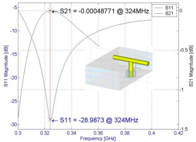
Figure 10: T-bar transition structure simulation results.
