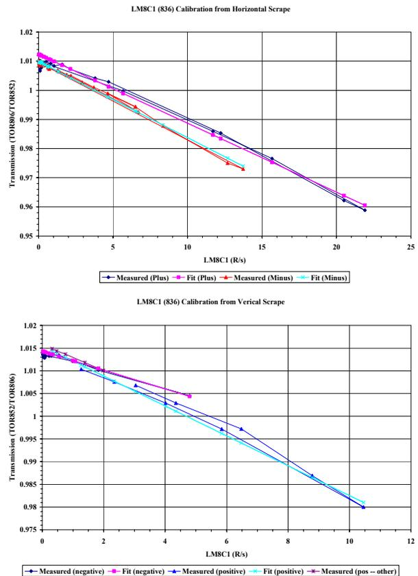
Figure 2: Calibration of loss monitor LM8C1 using transmission changes measured by beam toroids. Measurement from scraping horizontal edges above, vertical edges below.
