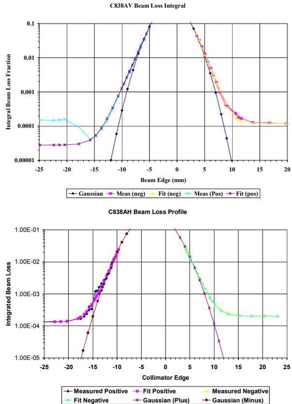
Figure 3: Integrated Beam Loss Profiles at C838A. Vertical profile shown above and horizontal profile shown below. The data is shown with the exponential fit described in Table 2 and a Gaussian profile integrated from the beam edge on each side. Gaussian width adjusted to visually match halo data.
