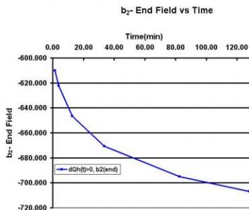
Figure 4: Calculated Value of  $b_2(\text{end})$  from the Measured Tune Drifts.
