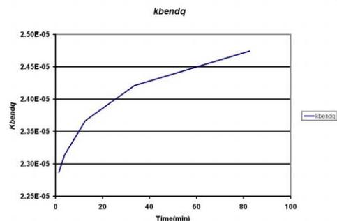
Figure 2: Calculated Value of  $kbendq$  from the Measured Tune Drifts.
