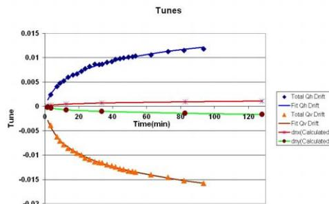
Figure 1: Tune Drift as a Function of Time on the 150GeV Front Porch, Measured and Calculated Values.
