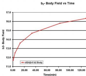
Figure 3: Calculated Value of  $b_2(\text{body})$  from the Measured Tune Drifts.
