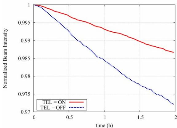
Figure 7: Normalized proton beam intensity, first two hours of an HEP store, simulated with LIFETRAC code.
