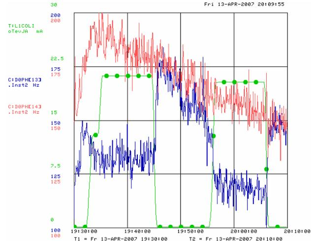
Figure 6: Dependence of proton loss rate of proton bunch #13 (C:DOPH[13]) and #14 (C:DOPH[13]) on TEL1 electron current (T:L1COLI).
