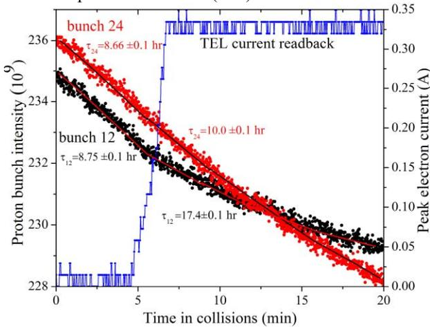
Figure 4: Effect of TEL2 on proton intensity decay.
