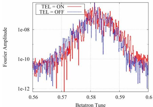
Figure 9: Proton vertical Schottky spectrum, computed with LIFETRAC code.
