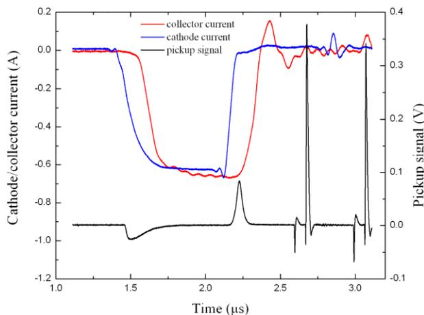
Figure 4: Cathode (blue) and collector (red) currents measured by current transformers. The artifacts on the right hand side are caused by the instrumentation. Pickup signal (black) featuring the electron pulse, two proton and two antiproton bunches. For clarity the electron pulse is shown timed to the abort gap where no bunches are present. The scope bandwidth was intentionally set to 20MHz to reject high frequency noise and limit bunch signal amplitude.
