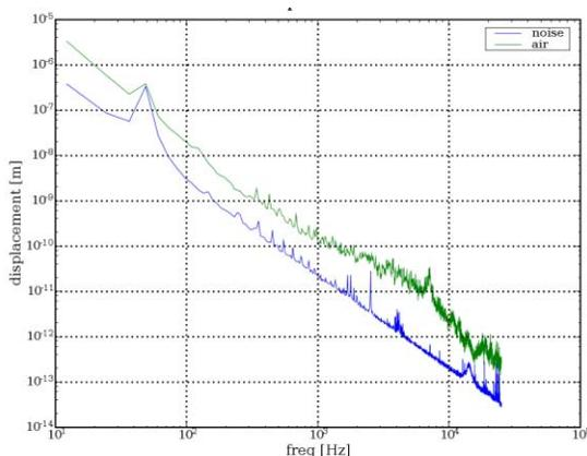
Figure 7: Spectrum of the piezo-accelerometer displacement signal induced by an airflow in the beam screen cooling channel.
