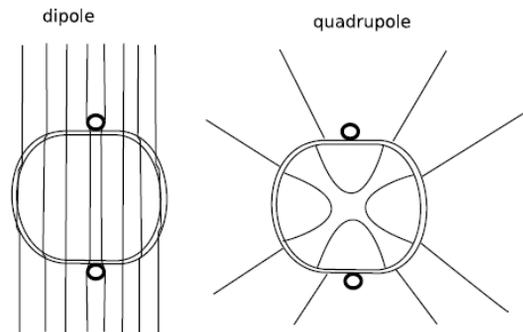
Figure 1: “Frozen” magnetic field lines in the LHC beam screen with shape oscillations (dip), and vibrations (quad).
