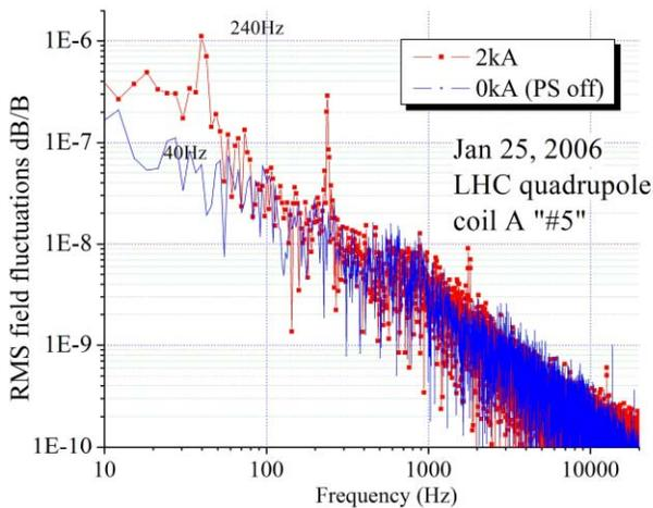
Figure 3: Signal from coil #5 placed in a SC MPY quadrupole at 2 kA.
