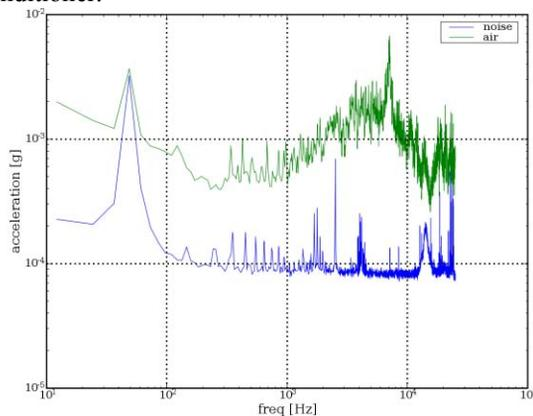
Figure 6: Spectrum of the piezo-accelerometer signal induced by an airflow in the beam screen cooling channel.
