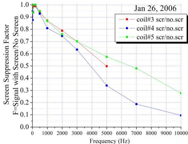
Figure 5: Additional field suppression by beam screen versus frequency.
