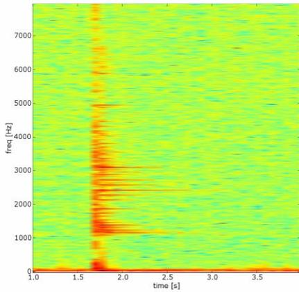
Figure 2: Spectrogram of the signals induced by hitting a beam screen immersed in a 700 Gauss B-field, illustrating the resonance frequencies of the beam screen sample.
