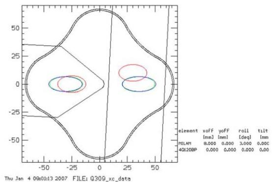
Fig. 7 The aperture at the MI injection Lambertson.
