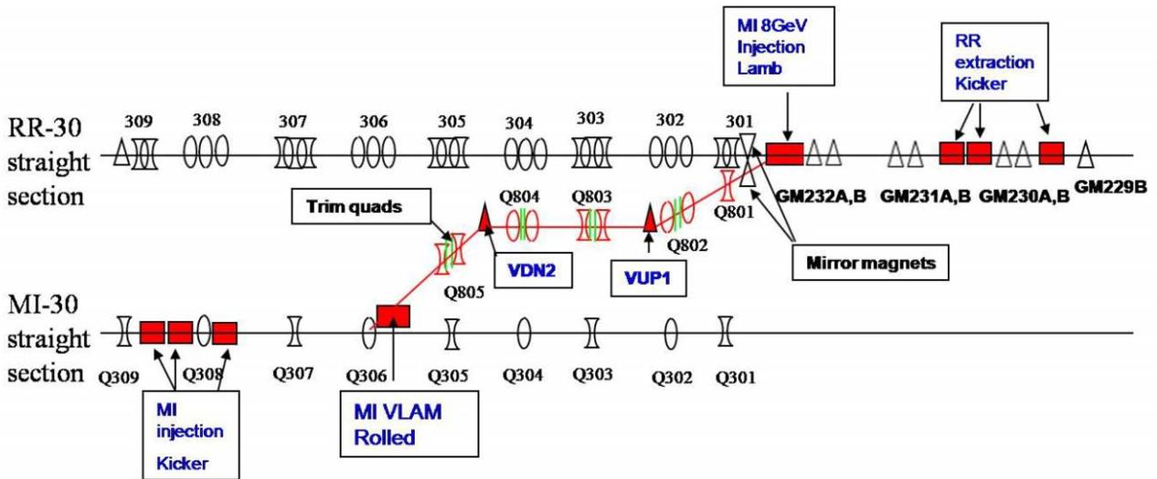
Fig. 2 Cartoon of extraction line, including RR and MI 30 straight section.
