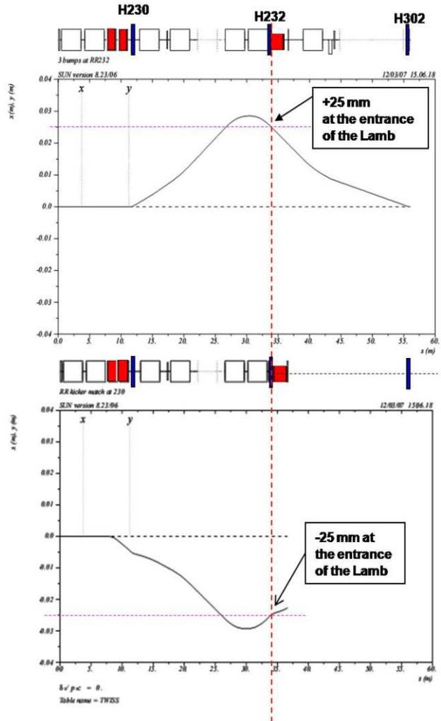
Fig. 4 Trajectories of circulating and extracted beam. The red blocks represent kicker modules. The blue blocks are 3 correctors.
