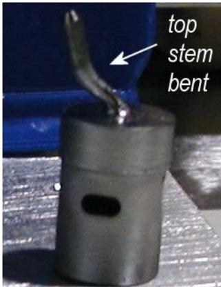
Figure 3: Tantalum oven's top stem bent after operation at 300 amps in high magnetic fields.
