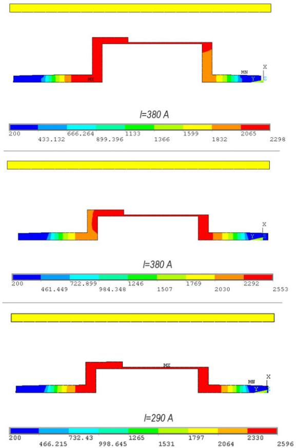
Figure 4: Temperature profiles of original size tungsten oven (top), new size tungsten oven (middle), and new size rhenium oven (bottom). All temperatures are Celsius. (Note that the color scale is different for all three profiles).
