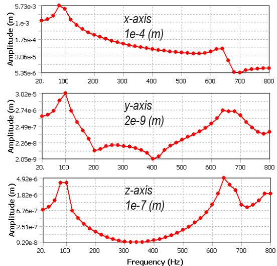
Figure 5: Amplitude harmonic response of oven system for the frequency range 0-800 Hz.
