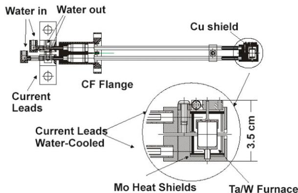
Figure 1: Compact LBNL high temperature oven.
