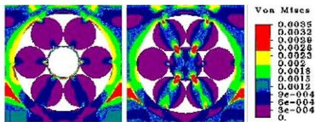
Figure 3: Von Mises strain in structured cable loaded vertically with 100 MPa: a) hollow spring tube in center; b) solid strand in center.
