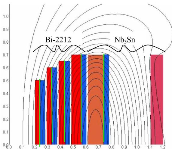
Figure 5: 35 T solenoid, 20 cm bore radius, with reverse winding: structured-cable windings (tan); stress shells (blue); expansion bladders (green). Dimensions in m.
