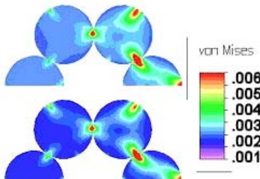
Figure 6: Von Mises strain distribution in inner shell at full field: a) innermost turn; b) outermost turn.
