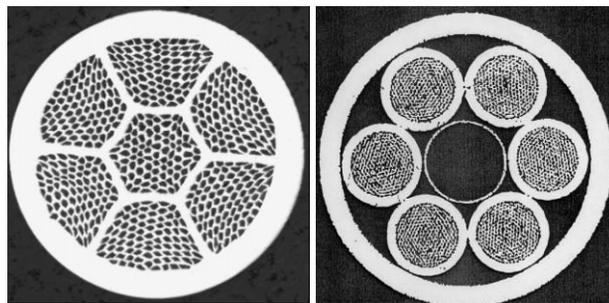
Figure 1: Bi-2212 strand and cable: a) Current high-performance Bi-2212 strand from OST; b) structured cable made using earlier strand.
