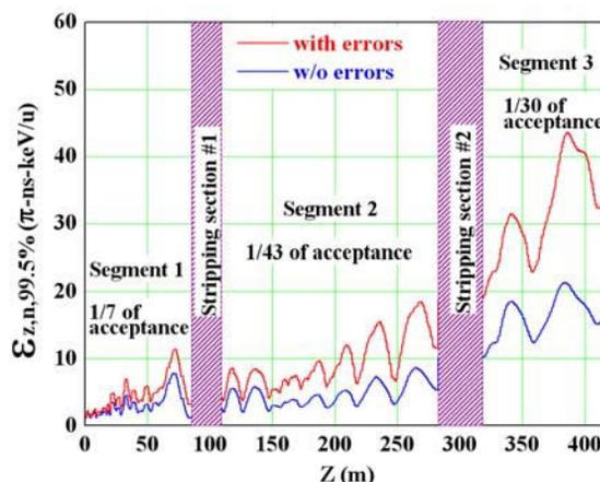
Figure 4: The longitudinal emittance evolution along the superconducting linac for uranium beam with (red) and without (blue) errors.
