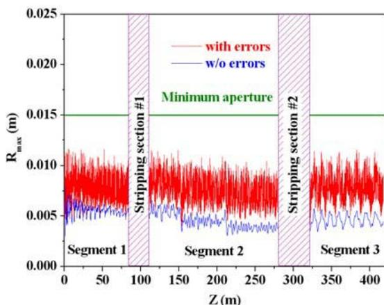
Figure 3: Beam envelopes of a multi-charge-state uranium beam without (blue) and with (red) errors along the driver linac. The minimum linac aperture is also indicated.
