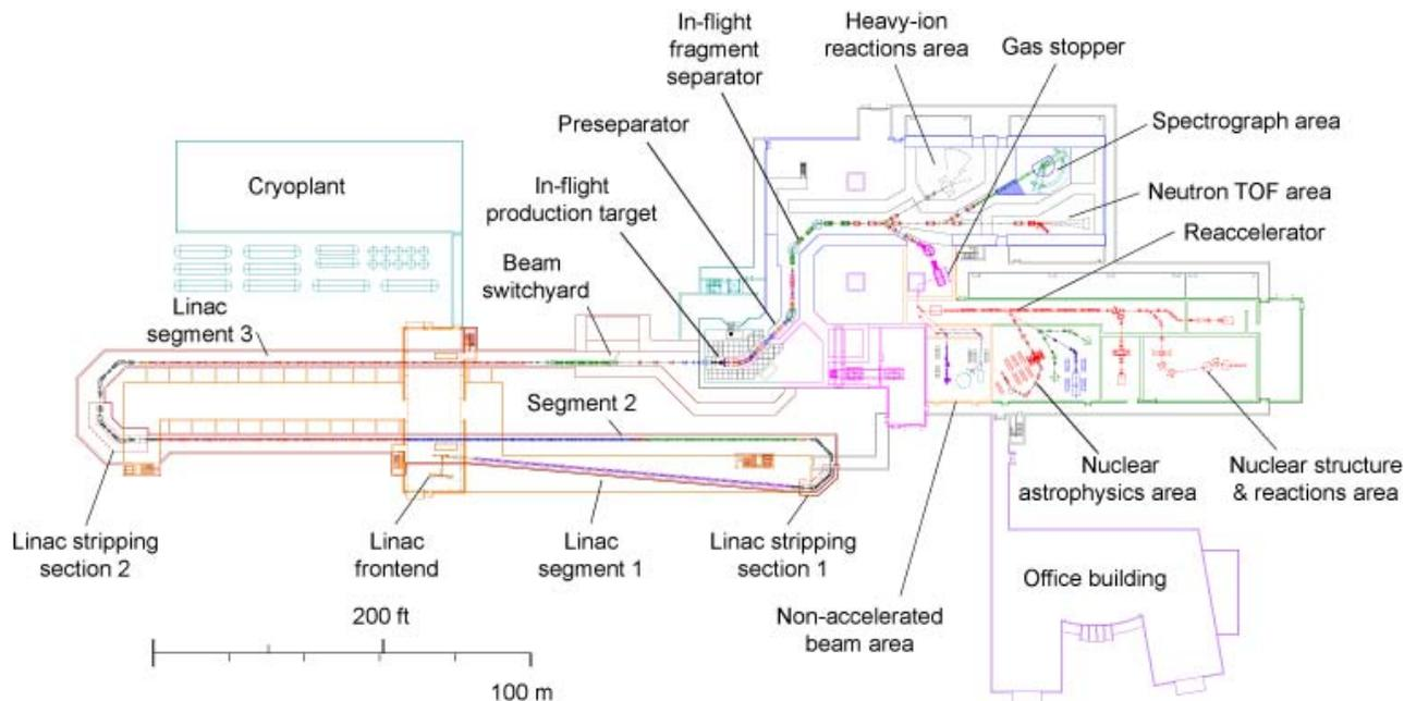
Figure 1: Layout of the accelerator complex and experimental areas. The driver linac consists of a room temperature front end and three superconducting linac segments, separated by two beam-stripping sections. The driver linac is designed to deliver up to 400 kW uranium beam power on a production target. Also shown is the reaccelerator linac, designed to deliver radioactive ions with energies in the range of 0.5 to 12 MeV/u.
