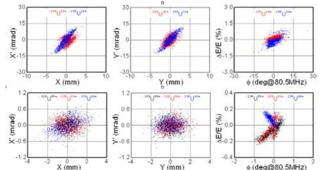
Figure 2: Phase space plots of sampled multi-charge-state uranium beam at the entrance (top) and the exit (bottom) of the superconducting linac.
