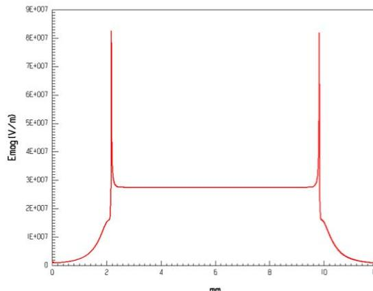
Figure 2: Magnitude of the electric field along the interface of SiC and indium solder meniscus for Case 1.
