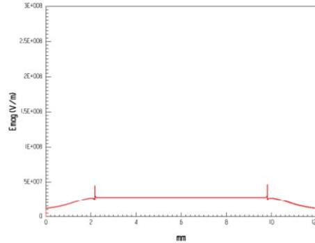
Figure 5: Magnitude of the electric field along the interface of SiC and indium solder meniscus for the case with nanoparticle composite filler.
