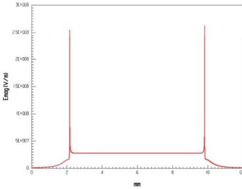
Figure 3: Magnitude of the electric field along the interface of SiC and indium solder meniscus for Case 2.
