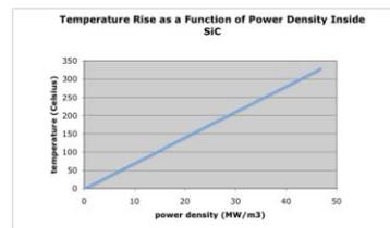
Figure 11: Peak temperature rise as a function of power density inside SiC after 100 seconds.
