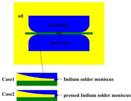
Figure 1: Two-dimensional configuration of a SiC switch. The bottom pictures show an enlarged view of the area between the electrode and SiC layer.
