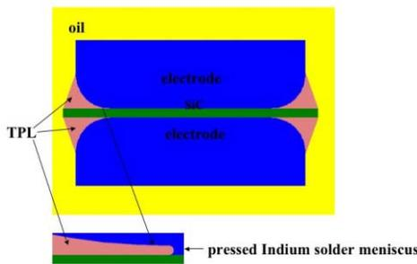
Figure 4: Two-dimensional configuration of a SiC switch with the nanoparticle composite filler. The bottom picture shows an enlarged view of the area between the electrode and SiC layer.
