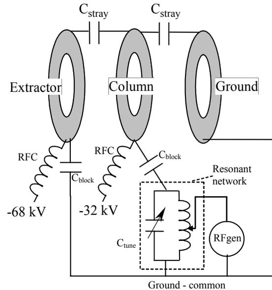
Figure 1: Schematic of prototype buncher circuit incorporated into HVDC column.
