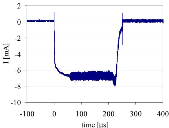
Figure 2: H- beam pulse ( $\sim 7$  mA) as measured with ISTS Faraday cup. RF bunching voltage applied  $\sim 60$   $\mu$ s after the start of beam pulse and remaining on for  $\sim 400$   $\mu$ s.
