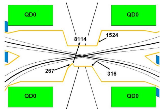
Figure 3: The mask tip is 3 mm in from the 10 mm radius beam pipe. This is the only surface that is inside the detector beam pipe so the overall masking design is quite open and has no obvious cavities for trapping higher-order-mode (HOM) power.
