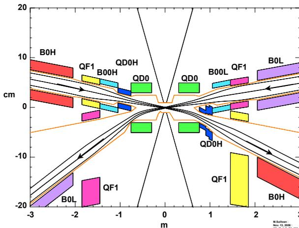
Figure 2: Closer view of the final focus magnets. The dark blue blocks are the QD0H permanent magnets. The design is different on each side of the IP. The incoming side has a narrow beam aperture and hence can be designed as a cylinder. The outgoing beam line for the HER has to accommodate the outgoing synchrotron radiation fan as well as the outgoing HER beam.
