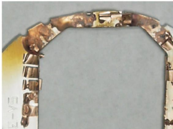
Figure 7: Damaged rf seal from a flex-flange connection.
