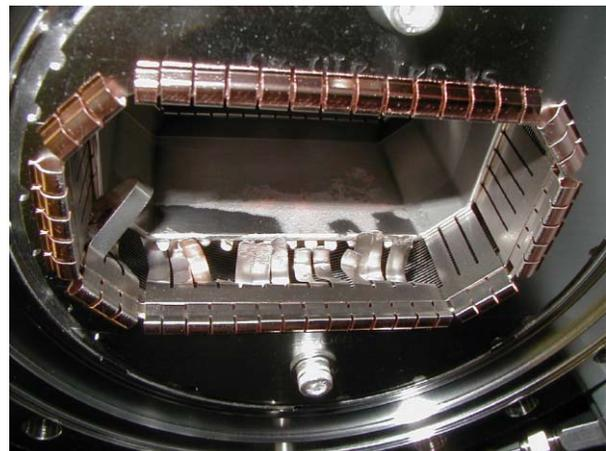
Figure 6: Damaged rf shield of a bellows unit.
