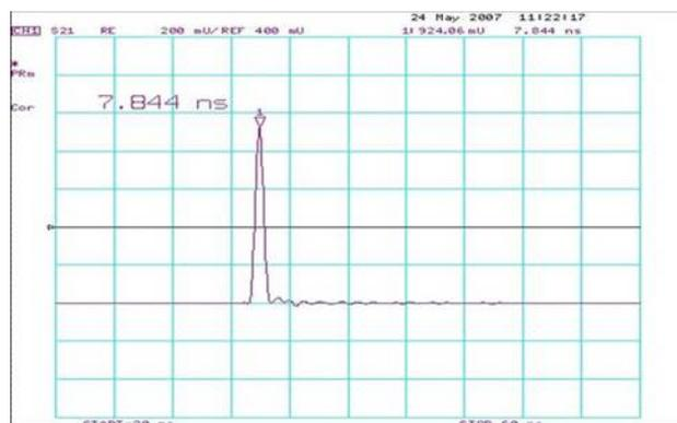
Figure 5. Results of the cold testing. Low voltage short pulse transmitted through the structure.
