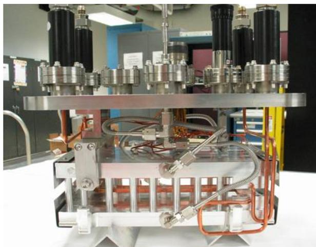
Figure 4. The new MEBT chopper deflector ready for installation.
