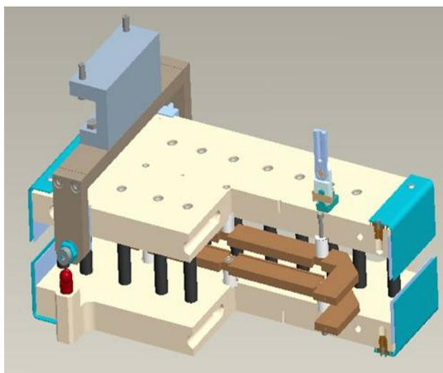
Figure 3. Layout of the new MEBT chopper deflector.
