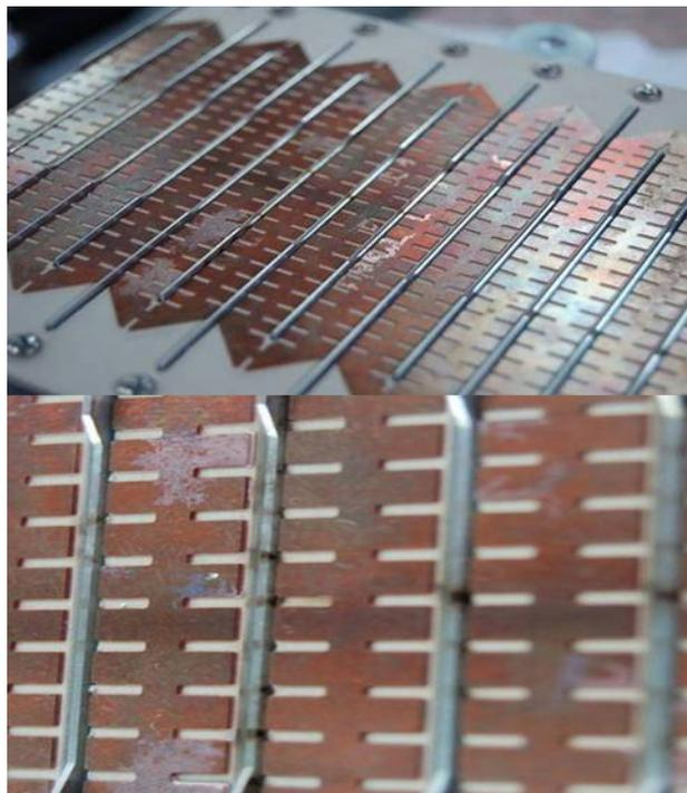
Figure 1. Photo of the damaged PCB structure of the original chopper deflector.
