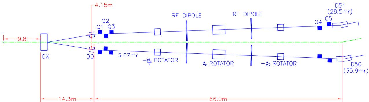
Figure 2: The schematic layout of RHIC spin flippers. The separate spin flippers in the two accelerators allows independent spin flipping in each ring.
