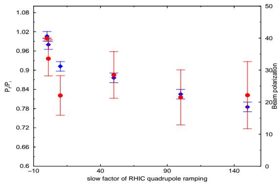
Figure 4: This plot shows the measured beam polarization after each resonance crossing as a function of the resonance crossing rate in units of RHIC quadrupole ramping slow factor. The higher the slowfactor, the longer it takes for the quadrupoles to ramp.
