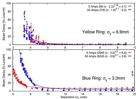
Figure 2: Beam loss rate as a function of vertical distance, in Yellow and Blue ring for experiment 2. The solid lines are power law fits to the respective data.
