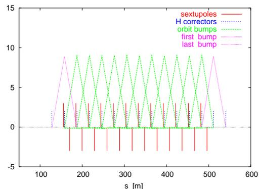
Figure 1: Corrector based bumps in the first arc.
