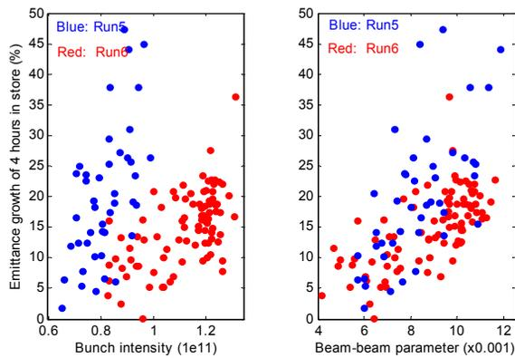
Fig. 6: The beam emittance growth of early 4 hours in store in Run 2005 and Run 2006 verses bunch intensity and beam-beam parameter.
