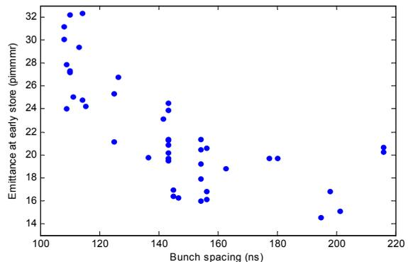
Fig. 5: Beam emittance at early store versus bunch spacing. The data are from Run 2005, with bunch numbers from 55 to 110.
