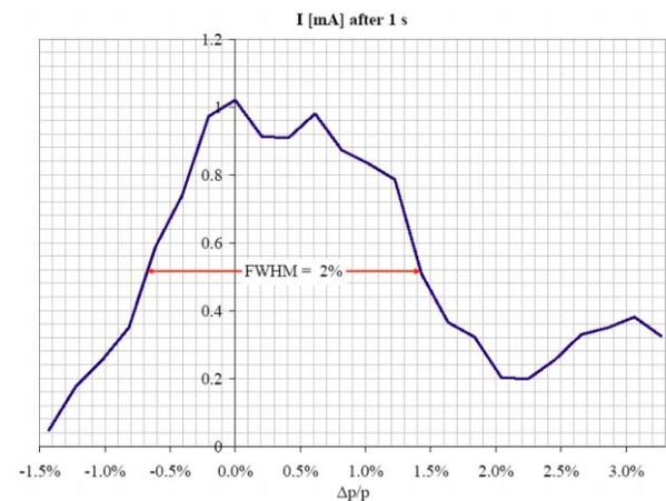
Figure 8: Circulating current after 1 s at 100 MeV.
