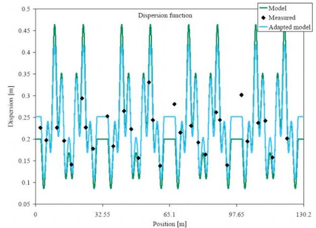
Figure 7: The dispersion function at 100 MeV.
