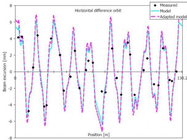
Figure 5: A horizontal difference orbit at 3 GeV.
