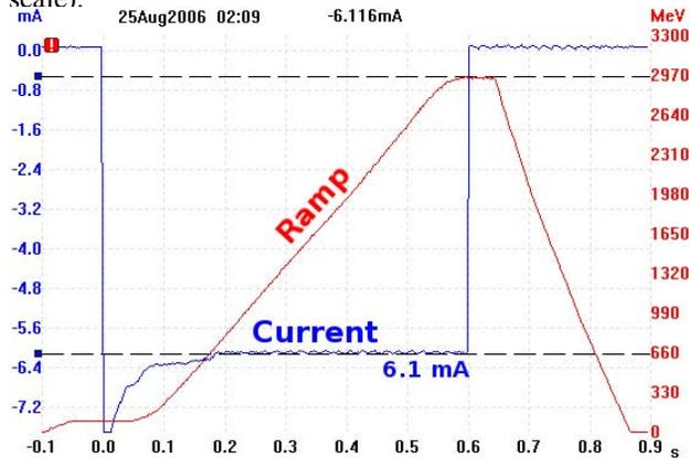
Figure 3: Circulating beam current (negative scale) during energy ramping (multi-bunch mode).
