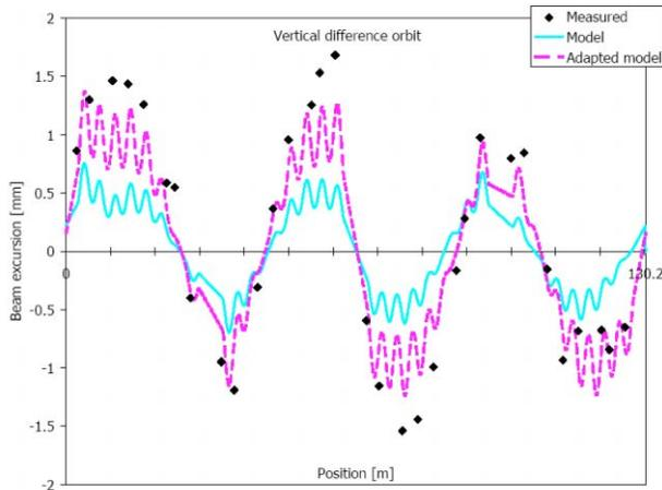
Figure 6: A vertical difference orbit at 3 GeV.
