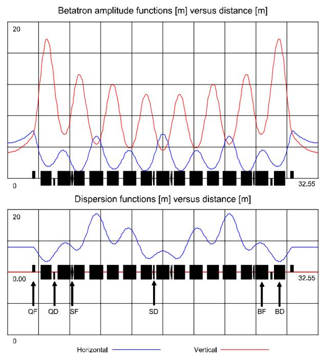
Figure 2: Betatron functions of the lattice.
