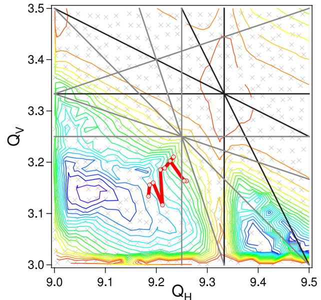
Figure 4: The tune (full red line) in the booster synchrotron during the energy ramp overlaid the simulated dynamic aperture. The black and grey lines are 3<sup>rd</sup> and 4<sup>th</sup> order resonances, respectively.
