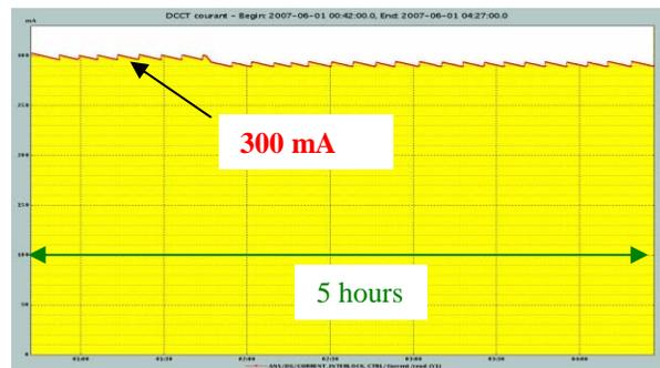
Figure 4: Frequent injection around 300 mA
