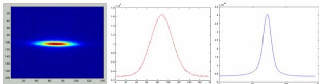
Figure 3: Image of the photon beam at its projections: horizontal (red) and vertical (blue).
