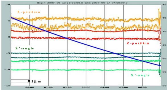
Figure 5: Angle and position evolution during an 8 hour user shift. The beam current variation is in blue.
