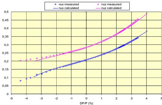
Figure 2: Tune shifts with energy: Comparison between measurement and modelling for the nominal lattice.
