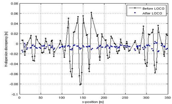
Figure 1: Horizontal dispersion function error before and after correction with LOCO.
