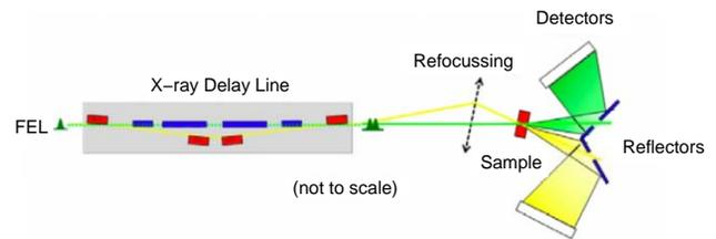
Figure 5: Optical layout of the time-resolved imaging experiment in the angular separation mode.
