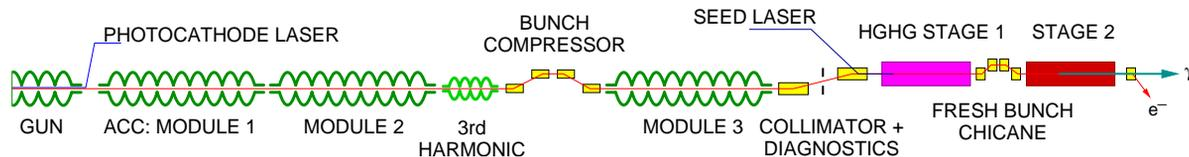
Figure 1: Layout of the main components of STARS.
