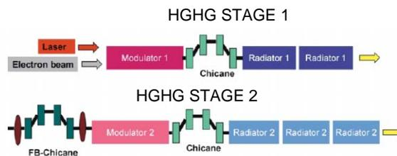
Figure 3: Schematic of the STARS two-stage HGHH cascade.
