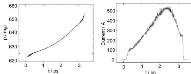
Figure 2: Simulated longitudinal phase space (left) and corresponding current distribution (right) of the electron bunches at the undulator entrance.
