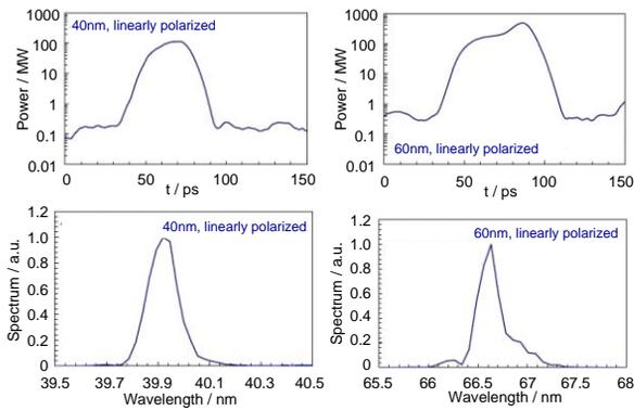
Figure 4: Temporal FEL pulse and spectra for STARS output radiation at 40 nm and 66 nm.
