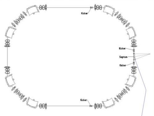
Figure 3: Lattice of MLS ring with pulsed elements
