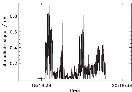
Figure 4: Synchrotron radiation of the first stored beam on 6th June (at 105 MeV electron beam energy) observed with photodiodes in the PTB diagnostics front end. From the photodiode responsivity a calibration factor of 0.3 nA photodiode current per 1  $\mu$ A electron beam current can be estimated.
