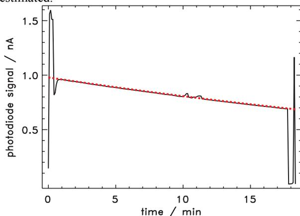
Figure 5: The measured beam lifetime ( $1/e$ ) at an electron energy of 105 MeV and at a stored electron beam current of several  $\mu$ A is approx. 1 h (red curve).
