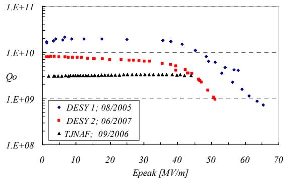
Figure 5: Cold (2K) RF-test results without lead coating.
