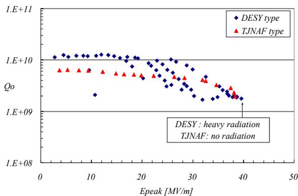
Figure 6: Cold (2K) RF-test results with lead coating.
