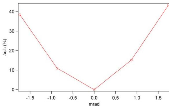
Figure 4: Emittance growth at the end of the injector due to a tilting of the solenoid in the horizontal plane.
