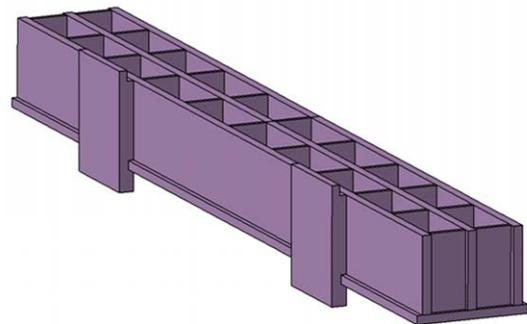
Figure 7: 3D model of backing beam without upper flange.
