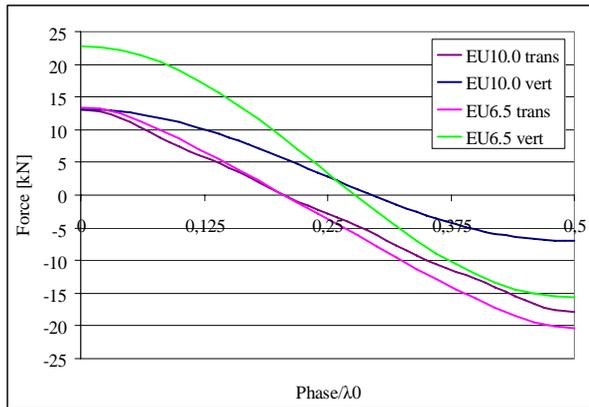
Figure 3: Vertical and transverse magnetic forces of the lower fixed array vs. phase for EU10.0 and EU6.5.
