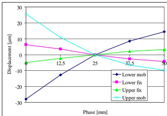
Figure 4: Measured transverse displacements of the four arrays of EU10.0 vs. phase.
