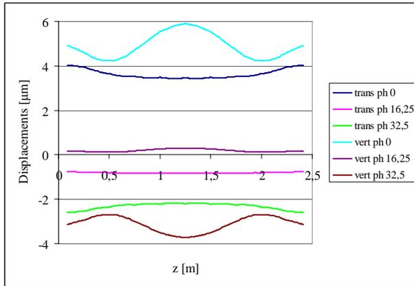
Figure 8: Lower fixed array transverse and vertical displacements vs. longitudinal position at different phase value.
