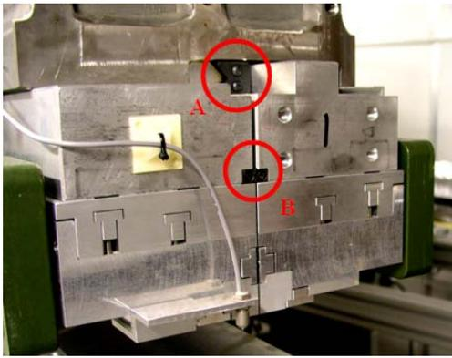
Figure 2: Linear bearing position: A is the main guide and B the small one.
