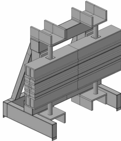
Figure 1: 3D model of an EPU carriage.
