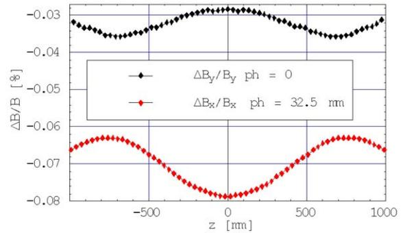
Figure 10: Peak field variation at zero phase and maximum phase.
