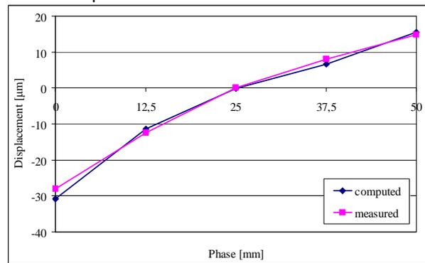
Figure 6: Mobile array: computed and measured transverse displacements.
