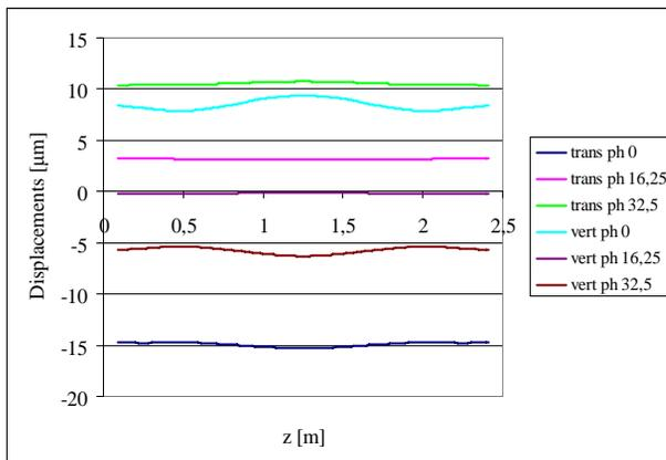
Figure 9: Lower movable array transverse and vertical displacements vs. longitudinal position at different phase value.
