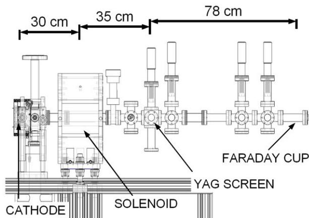
Figure 1: Measurement setup layout.
