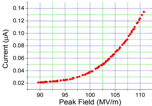
Figure 2: Darck current vs. accelerating RF field.
