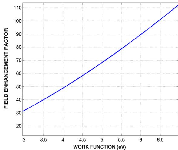
Figure 4: Field local enhancement factor vs. work function.
