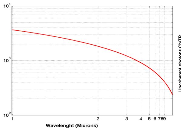
Figure 1: Uncoherent Cherenkov over uncoherent transition radiation photons vs. wavelength
