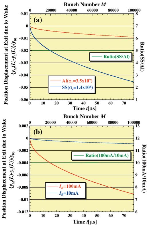
Figure 4: Position displacements at exit due to RW wake (a) for electric conductivities of pipes  $\sigma_c = 1.4 \times 10^6 \Omega^{-1} m^{-1}$  (SS: stainless steel) and  $3.5 \times 10^7 \Omega^{-1} m^{-1}$  (Al: aluminum) and (b) for the average currents  $I_b = 100$  mA and 10 mA with all the Q-magnets on as a function of time. Their ratios are also shown.
