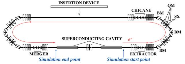
Figure 1: Layout of the planned test ERL in Japan
