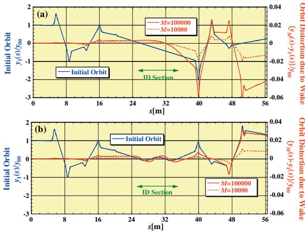
Figure 5: Initial orbits and orbit distortions due to the RW wake for  $M = 10000$  and  $100000$  ( $t = 7.7$  and  $77 \mu s$ ) with ID focusing strength (a)  $K_y = 0 m^{-2}$  and (b)  $K_y = 1 m^{-2}$  in a small-gap ID pipe at ID section.
