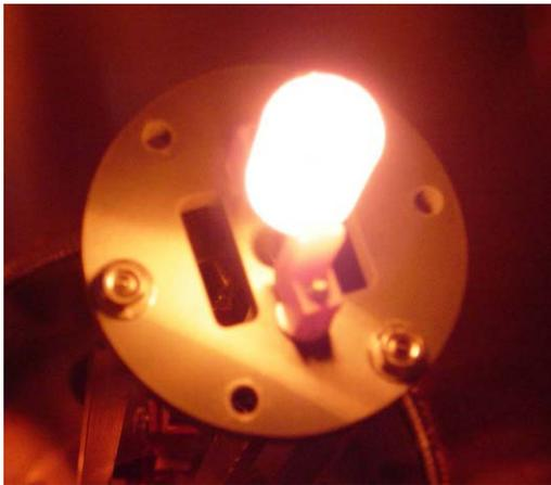
Figure 2: Operating graphite heater.
